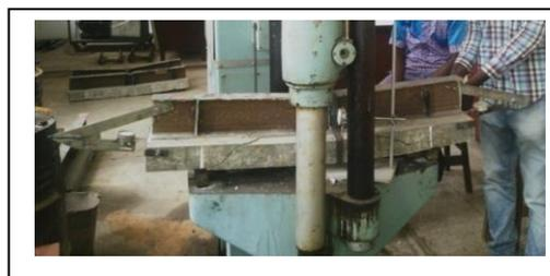
Fig. 4 One of the specimens under negative bending test
