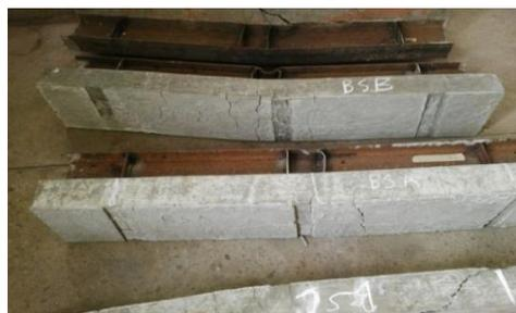
(b) Local buckling of the composite beams
