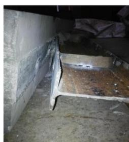
(a) Shear connector failure of BsD
